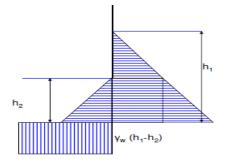
The maximum probable height outside the cofferdam during construction and the water height inside the cofferdam during various stages of construction need to be considered. These result in the net design pressure.
